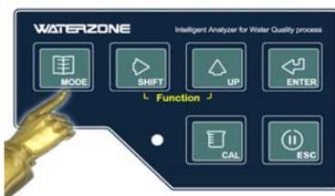
Figure 4-3 Membrane Keypad
